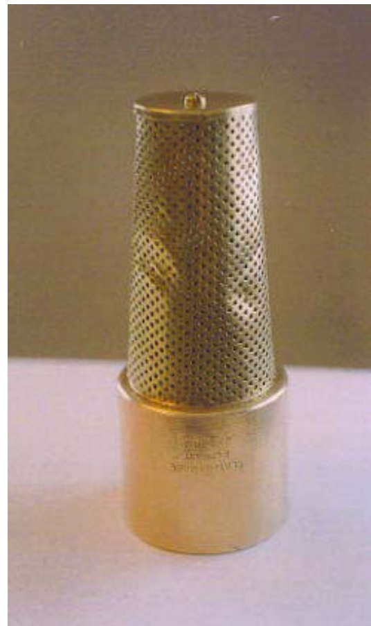
An early 1900's brass water strainer manufactured by Clayton Mark & Co. part number 2-5340. It too is now a part of the Marktown Preservation Society collection.
